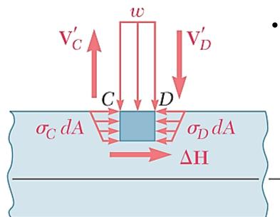
• The forces exerted on this element consist of vertical shearing forces  $V_C'$  and  $V_D'$ , a horizontal shearing force  $\Delta H$  exerted on the lower face of the element, elementary horizontal normal forces  $\sigma_C dA$  and  $\sigma_D dA$ , and possibly a load  $w\Delta x$ .
