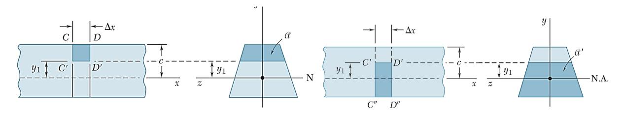
• This leads us to observe that the first moment Q of the portion a' of the cross section located below the line  $y=y_1$  is equal in magnitude and opposite in sign to the first moment of the portion a located above that line.
