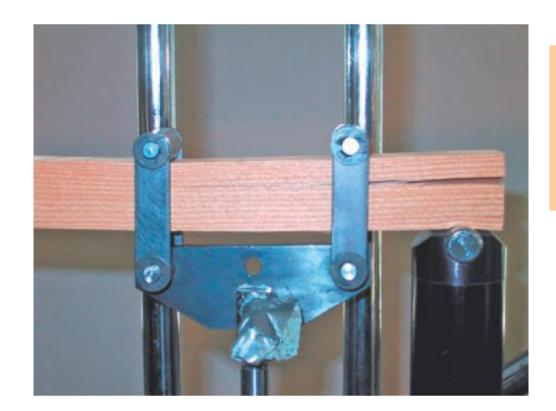
In timber beams, whose resistance to shear is weaker between fibers, failure due to shear occurs along a longitudinal plane rather than a transverse plane.
