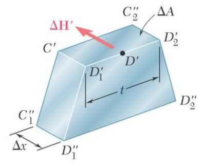
• Consider again a beam with a vertical plane of symmetry that is subjected to various concentrated or distributed loads applied in that plane. If, through two vertical cuts and one horizontal cut, an element of length  $\Delta x$  is detached from the beam.
