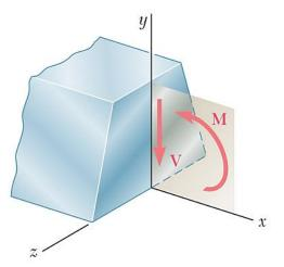
• Equation indicates that the average lateral shearing stress in any section is zero. However, this does not mean that the shearing stress  $\tau_{xz}$  is zero everywhere.
