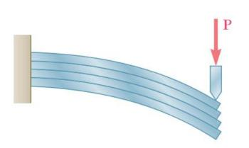
In contrast, if a couple M is applied to the free end of the same composite beam, the various planks bend into circular concentric arcs and do not slide with respect to each other. This <u>verifies the</u> <u>fact that shear does not occur in a beam subjected to pure</u> bending.
