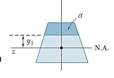
• where the integral extends over the shaded area A of the section located above the line  $y=y_1$ .
