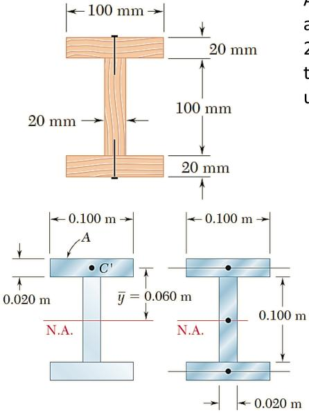
A beam is made of three planks, 20 by 100 mm in cross section, and nailed together. Knowing that the spacing between nails is 25 mm and the vertical shear in the beam is V = 500 N, determine the shearing force in each nail. Determine the horizontal force per unit length q exerted o the n lower face of the upper plank.
