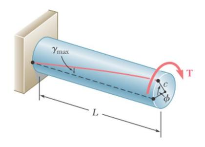
•  $\phi = \frac{TL}{JG}$  can be used for the angle of twist only if the shaft is homogeneous (constant G), has a uniform cross section, and is loaded only at its ends. If the shaft is subjected to torques at locations other than its ends or if it has several portions with various cross sections and possibly of different materials, it must be divided into parts that satisfy the required conditions.
