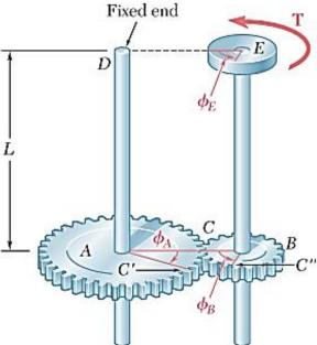
What torque should be applied to the end of the shaft to produce a twist of 2°? Use the value G = 77 GPa for the modulus of rigidity of steel.
