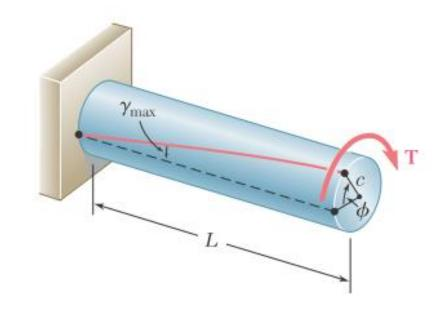
• But in the elastic range, the yield stress is not exceeded anywhere in the shaft. Hooke's law applies, and  $\gamma_{max} = {}^{\tau_{max}}/_{G}$ .
