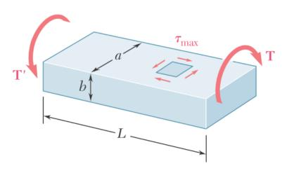
The maximum shearing stress occurs along the center line of the wider face and is equal to
