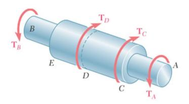
• For shaft AB shown in figure, four different parts should be considered: AC, CD, DE, and EB. The total angle of twist of the shaft (i.e., the angle through which end A rotates with respect to end B) is obtained by algebraically adding the angles of twist of each component part. Using the internal torque  $T_i$ , length  $L_i$ , cross-sectional polar moment of inertia  $J_i$ , and modulus of rigidity  $G_i$ , corresponding to part i, the total angle of twist of the shaft is
