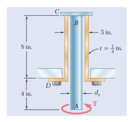
The solid spindle AB has a diameter  $d_s$  =1.75 in. and is made of a steel with G=11.2x10<sup>6</sup> psi and  $\tau_{all}$  =12 ksi, while sleeve CD is made of a brass with G=5.6x10<sup>6</sup> and  $\tau_{all}$  = 7 ksi. Determine (a) the largest torque  $\mathbf{T}$  that can be applied at A if the allowable shearing stress is not to be exceeded and if the angle of twist of sleeve CD is not to exceed 0.375°, (b) the corresponding angle through which end A rotates.
