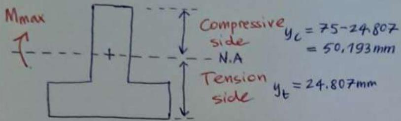
$$\star \sigma_t = \frac{M_{max} \cdot y_t}{I_x} = \frac{(2.25 \times 10^3)(24.807 \times 10^{-3})}{(850.195 \times 10^{-9})} = 65.652 \times 10^6 \text{ Pa} \quad (5)$$
