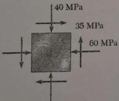
3. For the given state of stress, determine (a) the orientation of the planes of maximum in-plane shearing stress, (b) the maximum in-plane shearing stress, (c) the corresponding normal stress.
