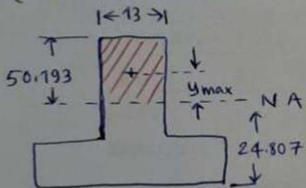
$$Q_{max} = (50.193)(13) \times \left(\frac{50.193}{2}\right) = 16.376 \times 10^3 \text{ mm}^3$$
