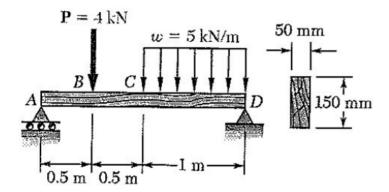
**9.48** For the timber beam and loading shown, determine (a) the slope at end A, (b) the deflection at the midpoint C. Use E = 12 GPa.
