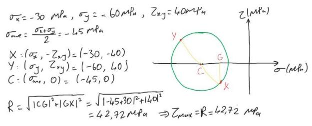
For the given state of stress, draw the Mohr Circle and determine the maximum shearing stress.
