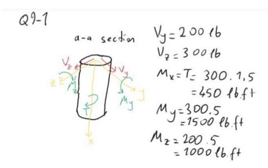
The 1-in.-diameter rod is subjected to the loads shown. Determine all forces and moment on the cross section of A-B plane.
