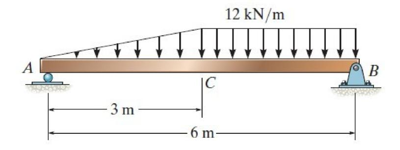
Q2) Draw the shear and bending-moment diagrams for each of the two segments of the compound beam.
