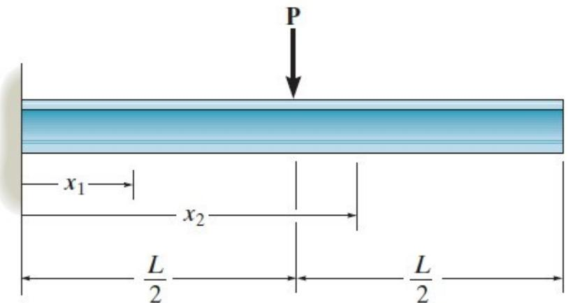
**12–13.** Determine the maximum deflection of the beam and the slope at  $A$ .  $EI$  is constant.
