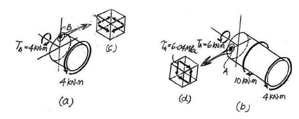
The solid shaft is fixed to the support at C and subjected to the torsional loadings shown. Determine the shear stress at points A and B on the surface, and sketch the shear stress on volume elements located at these points.
