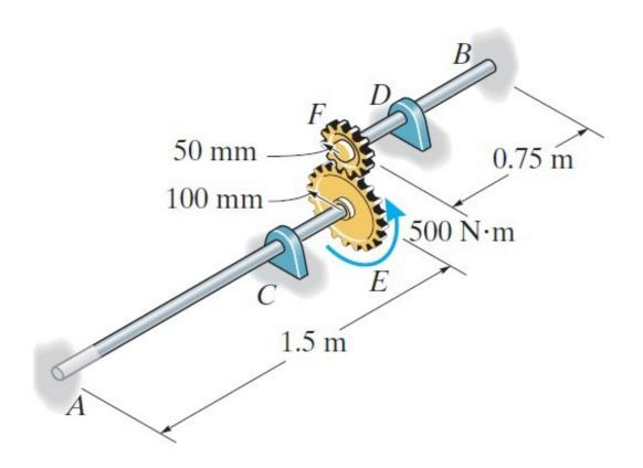
5-87. Determine the rotation of the gear at E in Prob. 5-86.
