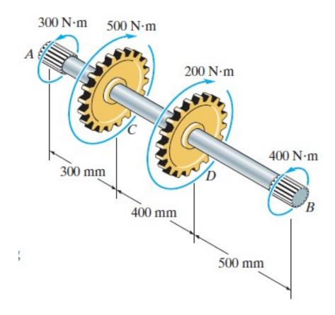
5–13. If the tubular shaft is made from material having an allowable shear stress of  $\tau_{\text{allow}} = 85 \text{ MPa}$ , determine the required minimum wall thickness of the shaft to the nearest millimeter. The shaft has an outer diameter of 150 mm.
