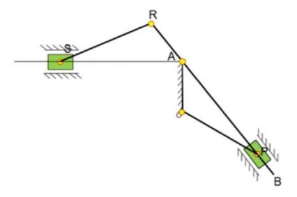
Figure below shows the configuration of a Whitworth Quick Return Mechanism. The lengths of the fixed link OA and the crank OP are 200 mm and 350 mm respectively. Other lengths are: AR = 200 mm and RS = 400 mm. Find the velocity of the ram using I-Center method when the crank makes an angle of  $120^\circ$  with the fixed link and rotates at 10 rad/sec.
