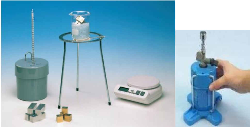
Fig. 1: Experimental set-up for determining the heat capacity of metals.
