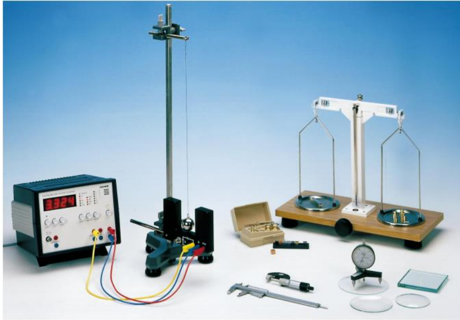
Fig. 1: Experimental set-up: Measurement of basic constants: length, weight, and time.
