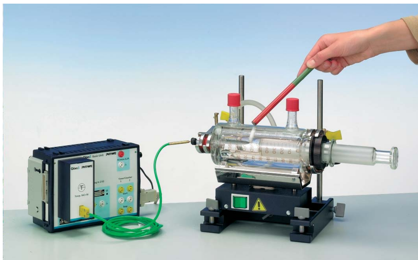
Fig. 1. Experimental set-up for Gay-Lussac's law
