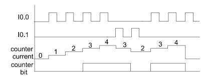
**P.3** Write a PLC program, using counters, to produce the waveforms given below at the output named Q=0.0 and Q0.1. Program must be in the form of ladder diagram.
