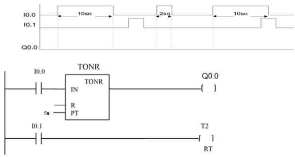
**P.3** Write a PLC program, using timers, to produce the waveforms given below at the outputs named Q0.0, Q0.1, Q0.2. The program must be in the form of ladder diagram.
