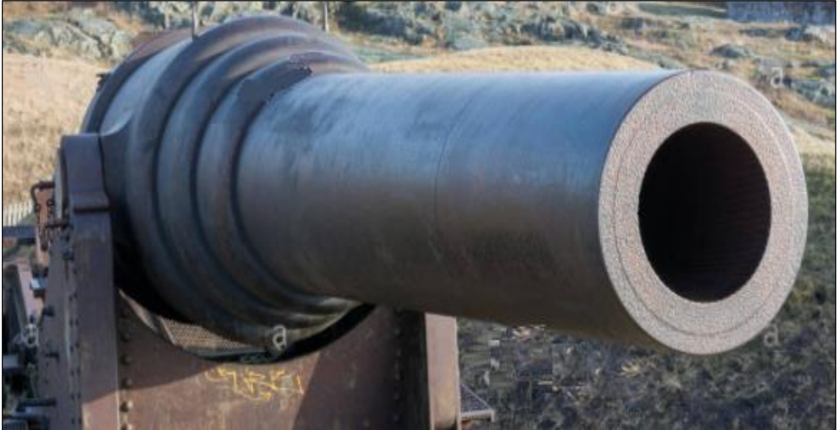
Figure 3 Press fitted cannon barrel
