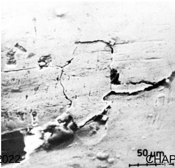
Surface failures due to contact stresses
