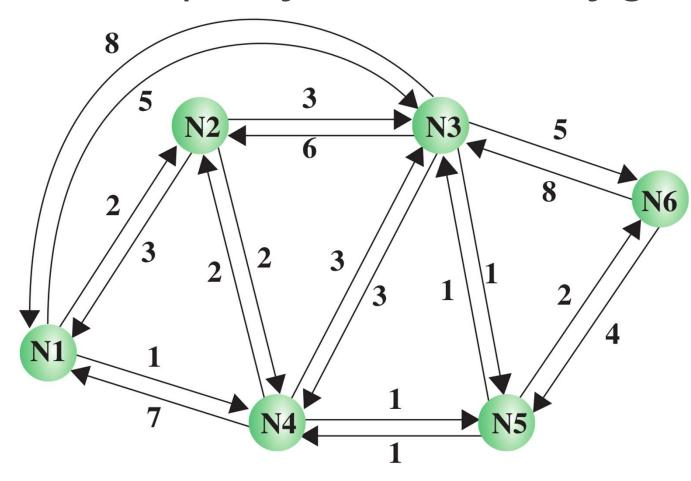
N1 to N6 are **nodes**, arrows are **links** with direction and the numbers on the links show the **costs**. Costs of full duplex data transfer may be different.
