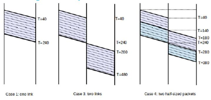
Bandwidth delay 200 µsec, per-link propagation delay 40 µsec
