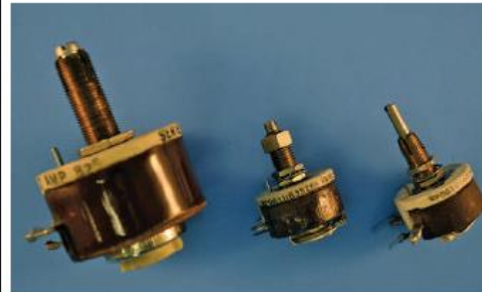
A rheostat is a variable resistor used to control current.
