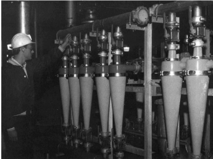
FIG. 18.7 Battery of hydrocyclones used for separation of germ from milled steeped corn. (Courtesy of Dorr-Oliver, Inc., Stamford, Connecticut.)
