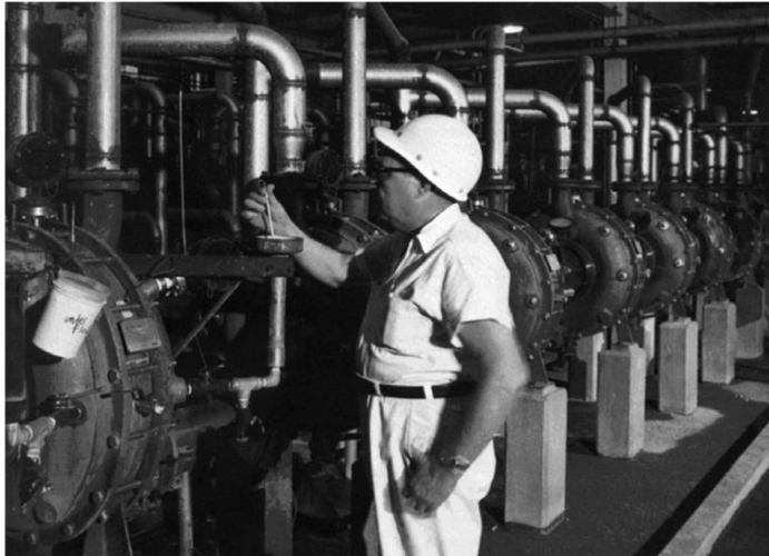
FIG. 18.11 Hydrocyclone starch washing and starch separating units. Each clamshell contains as many as 480 individual hydrocyclone tubes 10mm in diameter. (Courtesy of Dorr-Oliver, Inc., Stamford, Connecticut.)
