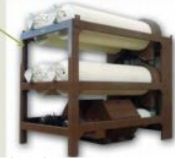
Trior-Intented cylinder (to separate broken kernel and foreing seed)
